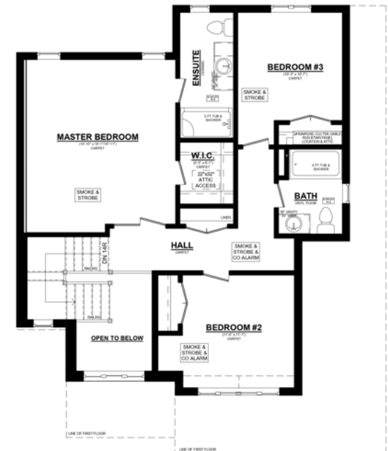
LIVINGSTON B 2ND FLOOR PLAN 908 SQ. FT. (DOES NOT INCLUDE 62 SQ. FT. OPEN TO BELOW) 8" CEILINGS ON 2ND FLOOR
