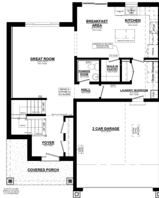
LIVINGSTON B MAIN FLOOR PLAN 939 SQ. FT. 8" CEILINGS ON MAIN FLOOR
