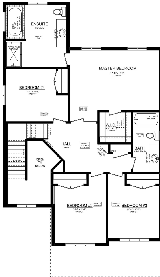
EDENBROOK 'A' 2ND FLOOR PLAN 1160 SQ. FT. (DOES NOT INCLUDE 134 SQ. FT. OPEN TO BELOW) 8' CEILINGS ON 2ND FLOOR
