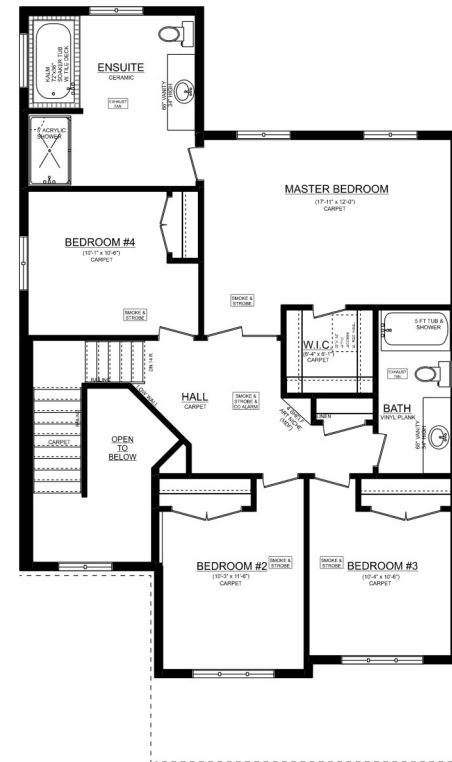
EDENBROOK 'A' 2ND FLOOR PLAN 1160 SQ. FT. (DOES NOT INCLUDE 134 SQ. FT. OPEN TO BELOW) 8' CEILINGS ON 2ND FLOOR
