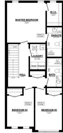
Ashton B UNIT #1 2ND FLOOR PLAN PLAN 910 SQ. FT. 8' CEILINGS ON 2ND FLOOR' CEILINGS ON 2ND FLOOR PLAN
