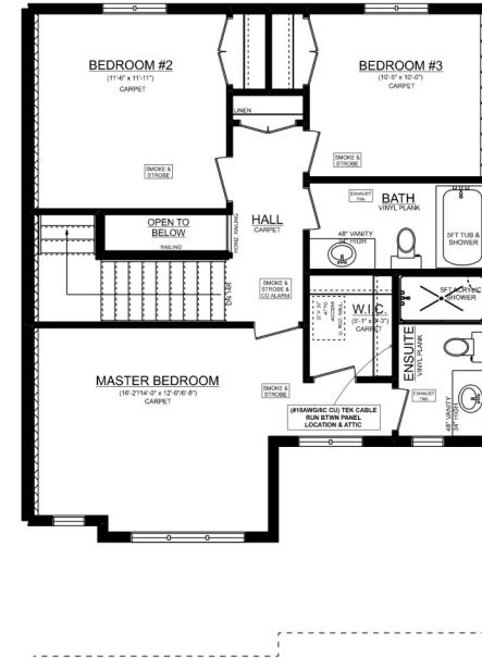
ELMWOOD 'B' UNIT #2 2ND FLOOR PLAN 8' CEILINGS ON 2ND FLOOR 775 SQ. FT. DOES NOT INCLUDE 75 SQ.FT OPEN TO BELOW
