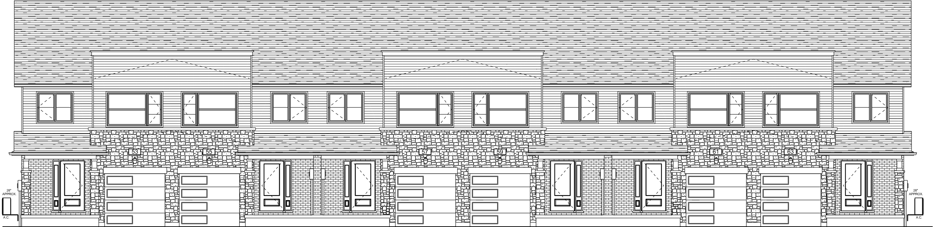
ELEVATION 'A' 8' CEILINGS ON MAIN FLOOR
