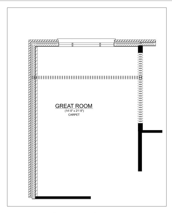
extend rear wall to make flush across the back of the home increasing the great room and basement size (adds 70sq ft to the home). Enlarge arch between Great Room and Breakfast Area to 10 ft. and add mechanical chase wall to great room side wall. Add roof to rear of home over extended Great Room. Add beams to hold up 2nd floor.
